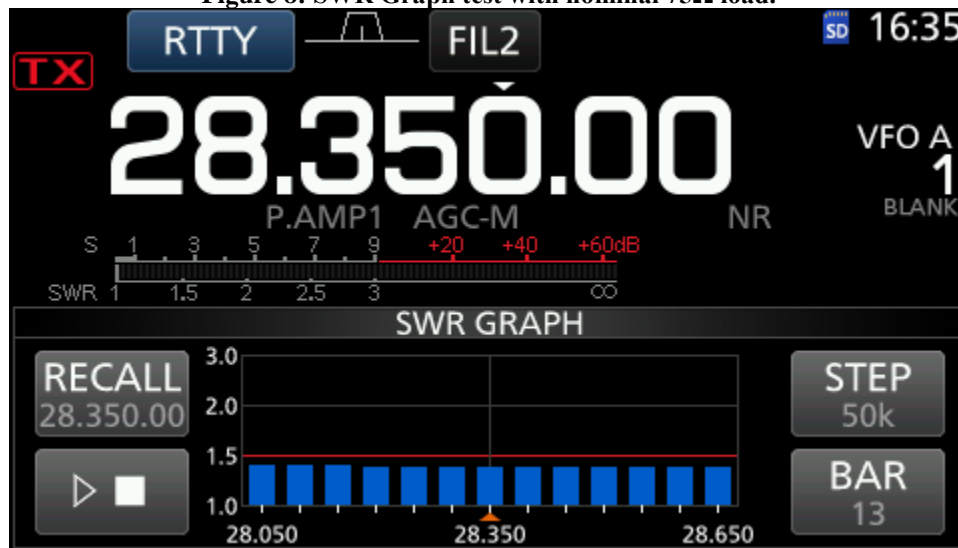
Figure 8: SWR Graph test with nominal 75Ω load.
