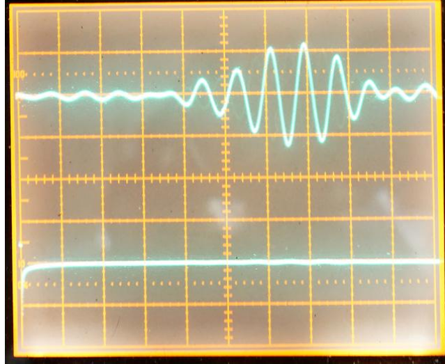
Figure 7: RX latency, 250 Hz SOFT CW filter. 2 ms/div.
